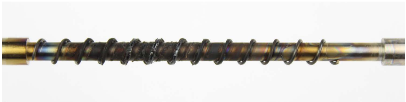
Figure 50: Conventional oil #4 TEOST MHT rod deposits
