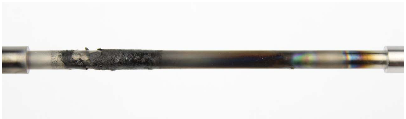
Figure 51: Conventional oil #4 TEOST 33C rod deposits
