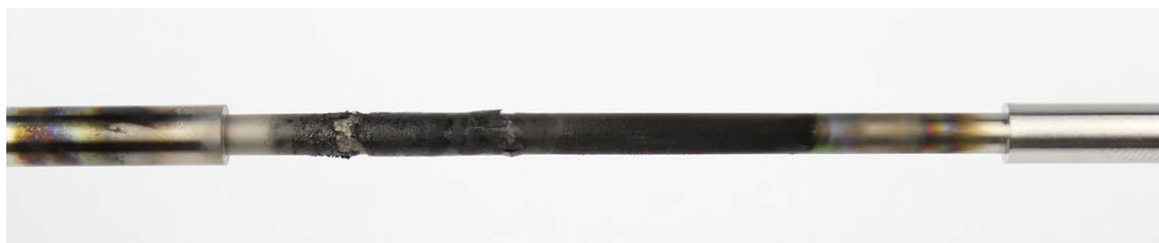
Figure 45: Conventional oil #1 TEOST 33C rod deposits
