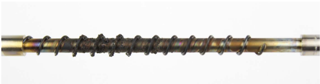
Figure 52: Conventional oil #5 TEOST MHT rod deposits
