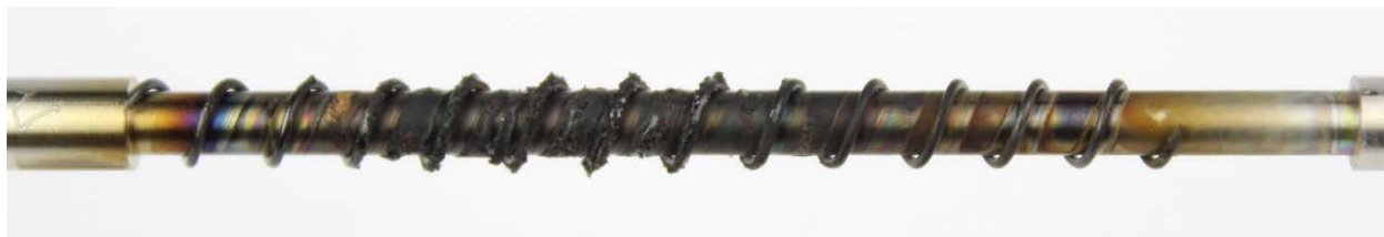
Figure 60: Synthetic oil #4 TEOST MHT rod deposits
