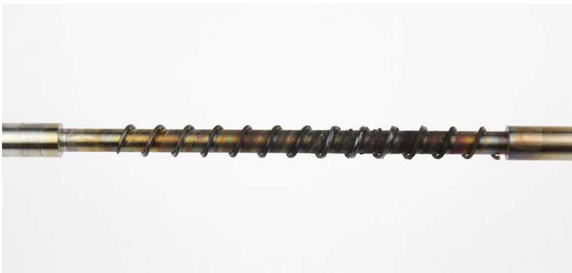
Figure 44: Conventional oil #1 TEOST MHT rod deposits
