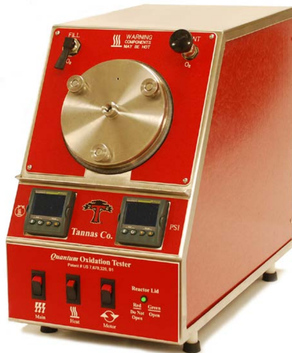
Figure 22: ASTM D4742 TFOUT instrument Image Source: AAA
