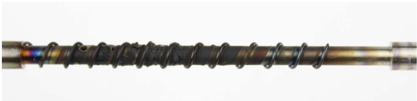
Figure 56: Synthetic oil #2 TEOST MHT rod deposits
