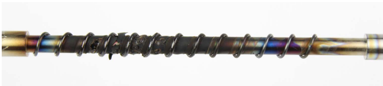
Figure 58: Synthetic oil #3 TEOST MHT rod deposits
