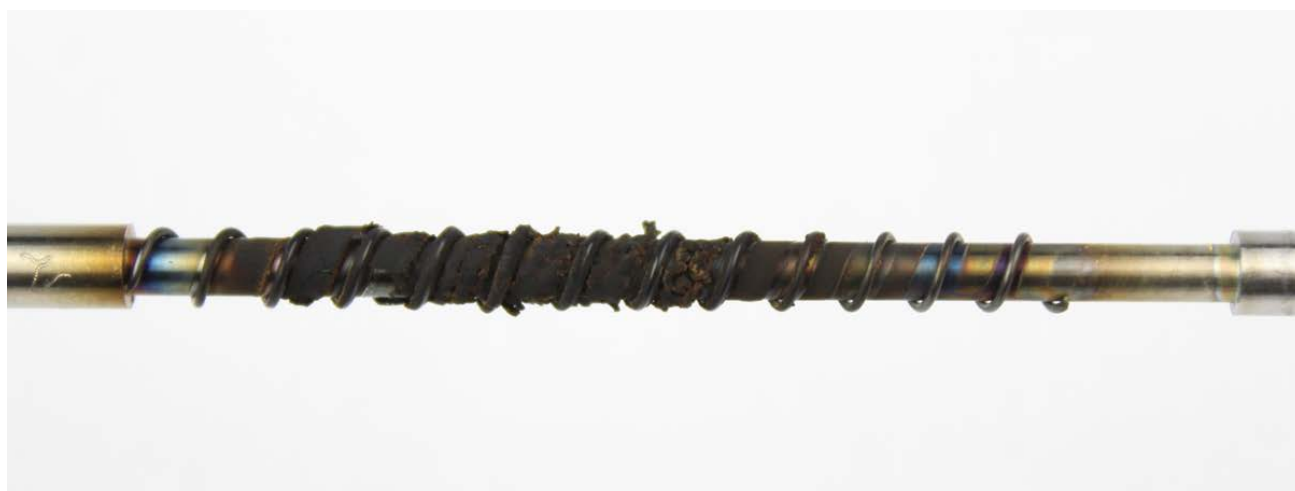
Figure 46: Conventional oil #2 TEOST MHT rod deposits
