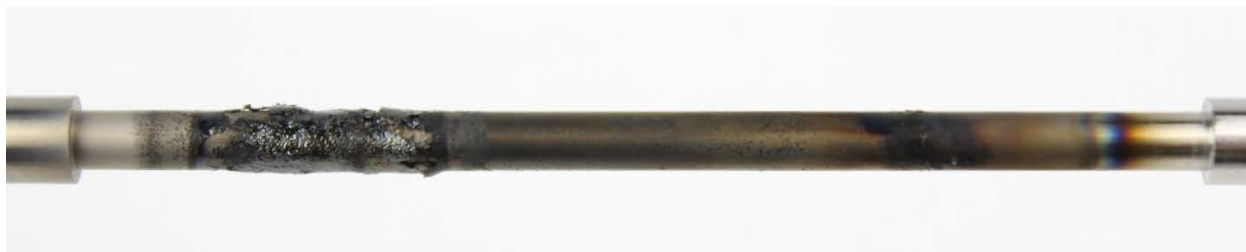
Figure 61: Synthetic oil #4 TEOST 33C rod deposits
