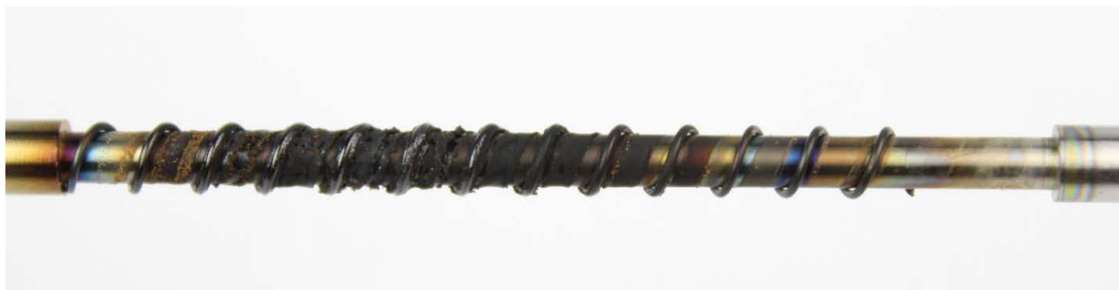
Figure 62: Synthetic oil #5 TEOST MHT rod deposits
