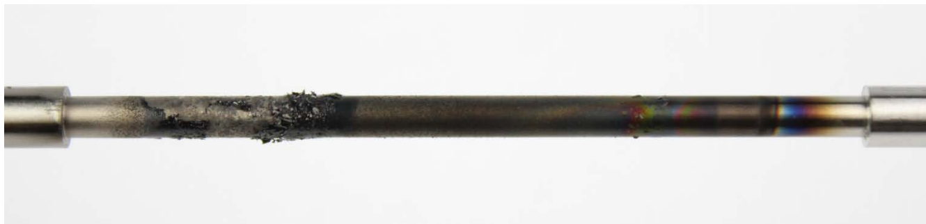
Figure 59: Synthetic oil #3 TEOST 33C rod deposits
