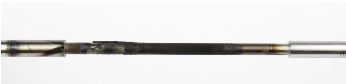
Figure 53: Conventional oil #5 TEOST 33C rod deposits
