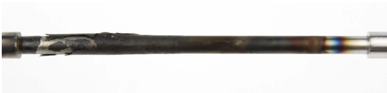
Figure 47: Conventional oil #2 TEOST 33C rod deposits
