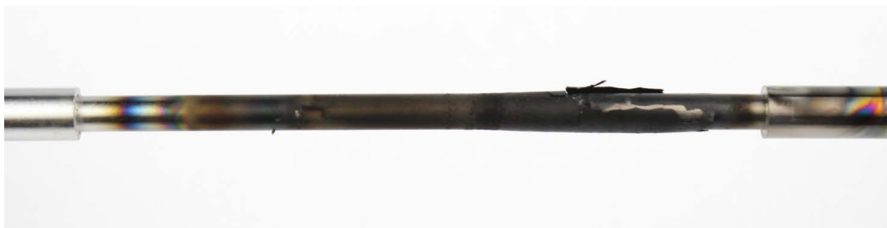
Figure 49: Conventional oil #3 TEOST 33C rod deposits
