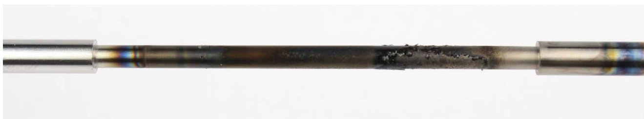
Figure 57: Synthetic oil #2 TEOST 33C rod deposits
