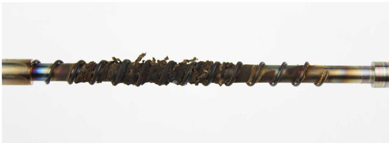
Figure 48: Conventional oil #3 TEOST MHT rod deposits
