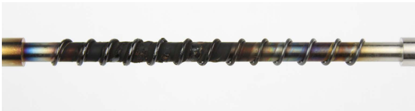
Figure 54: Synthetic oil #1 TEOST MHT rod deposits
