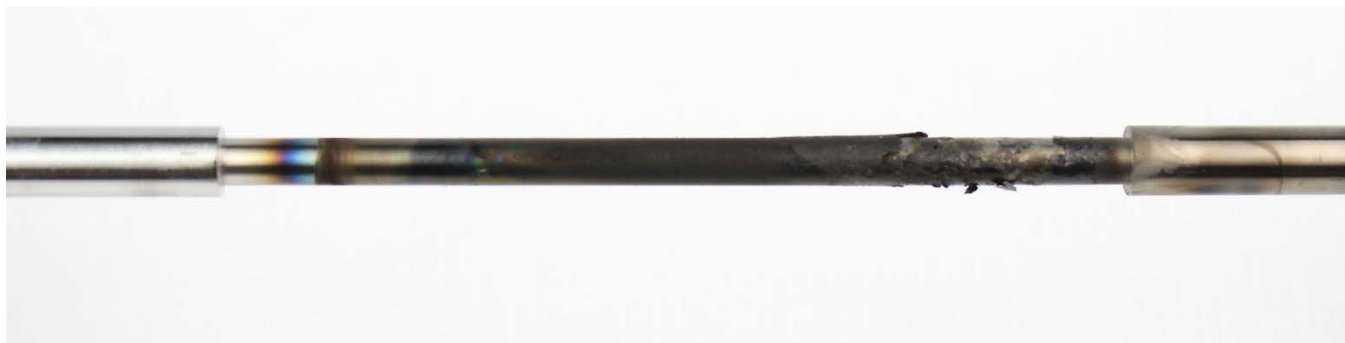
Figure 55: Synthetic oil #1 TEOST 33C rod deposits
