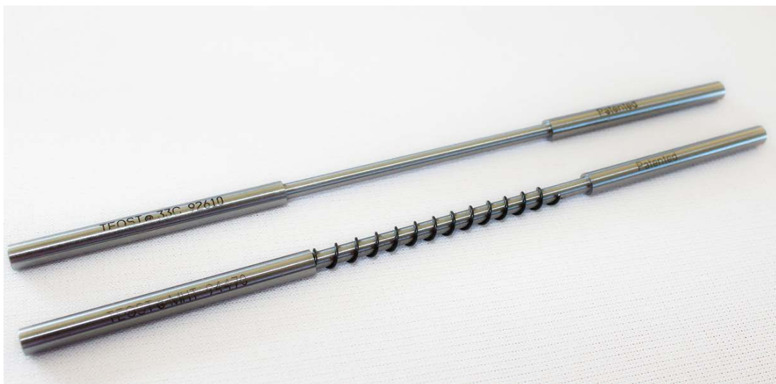
Figure 43: TEOST MHT & 33C depositor rods
