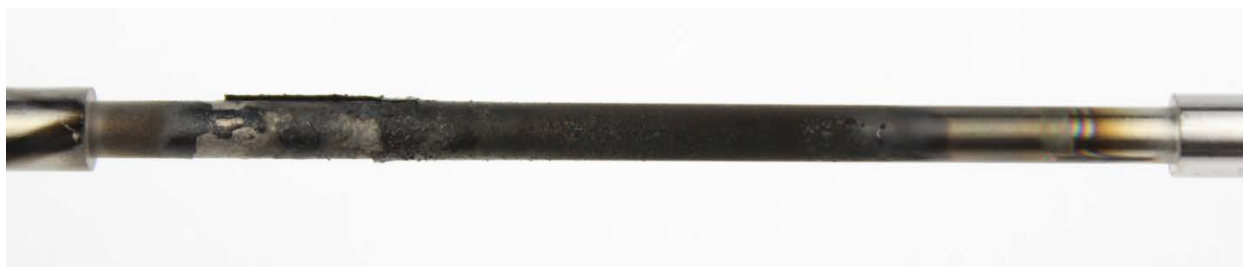
Figure 63: Synthetic oil #5 TEOST 33C rod deposits
